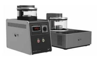
The Ion Sputter Coater allows for imaging of nonconductive samples in high vacuum mode for the highest resolution imaging. Sputter coaters increase conductivity by coating the test specimen with a few nanometer thick metal film of Au or Pt. The higher conductivity increases the amount of secondary electron generation and creates higher resolution images. \* Coating Target: Au or Pt
